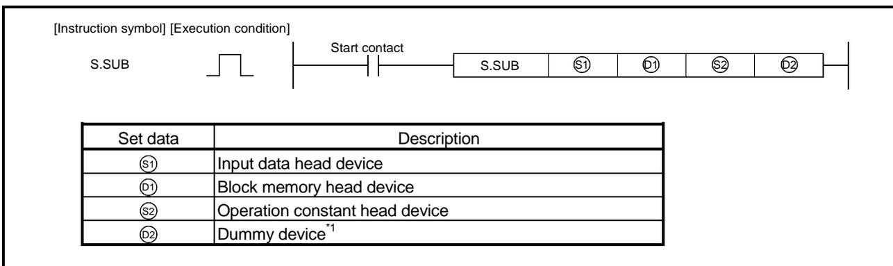
\*1: Special register SD1506 can be specified as a dummy device.
