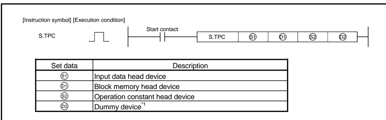
\*1: Special register SD1506 can be specified as a dummy device.
