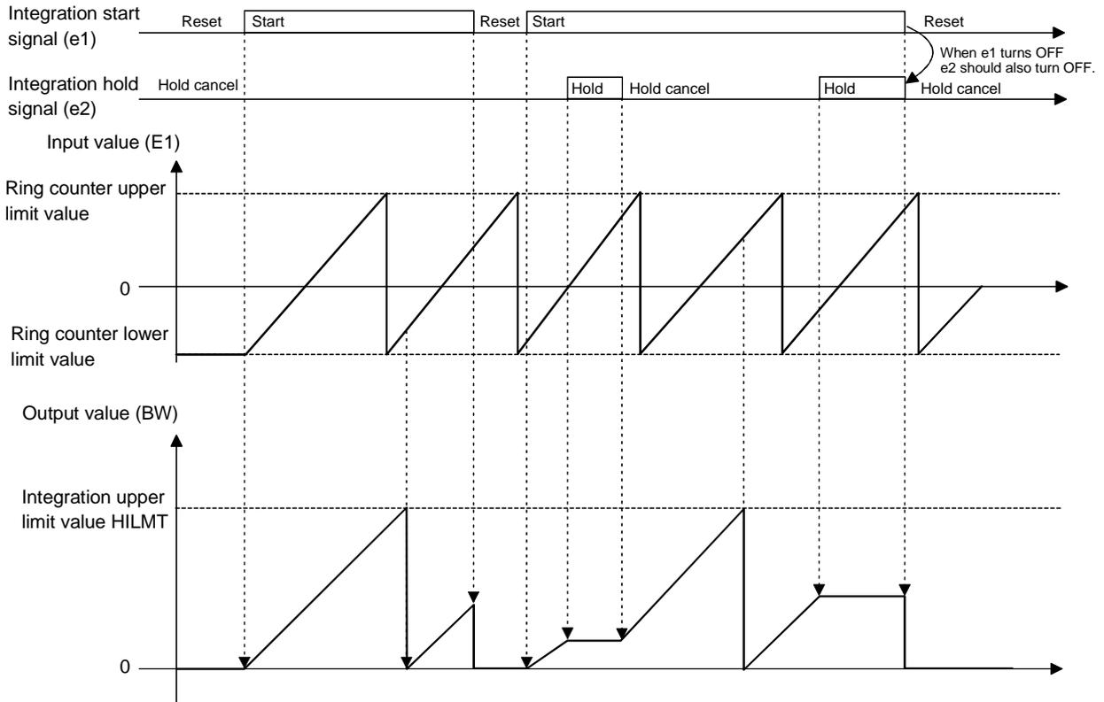
(2) Operation performed when the integration pattern is set to "integrated value is retained at the integration upper limit value when the upper limit value is exceeded"
