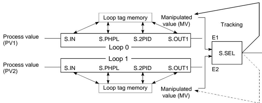
Example) When the S.SEL instruction uses the input value E1 and E1 uses the upper loop (loop 0) MV, the S.SEL instruction's MV is tracked to loop 0's MV. The setting that conducts Tracking is shown below.
