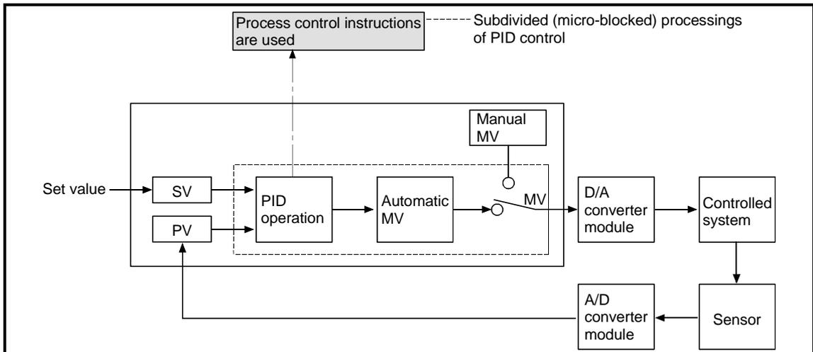
Fig. 1.1 Example of application to process control
