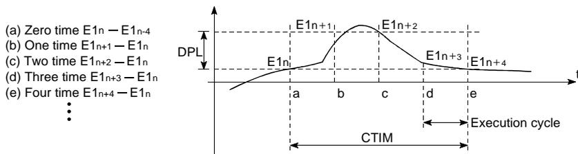
(b) The change of the input data is compared with the change rate alarm value (DPL) in each execution cycle ( $\Delta T$ ).
