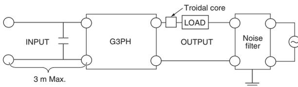
Recommended Capacitor (Film Capacitor) Input: 0.1  $\mu$ F, 250 VAC
